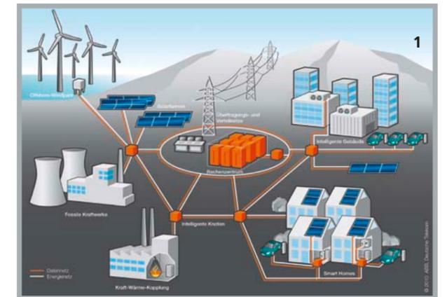
energy turnaround, there is an increased need for long-term energy storage and a control system, which together offset the differences between fluctuating weather-dependent generation and power consumption.
