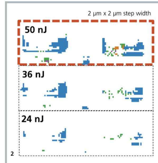
In Figure 2, the white dotted section roughly outlines one of the data channels of the Digital Isolator 14850 (step width in x and y direction 5 µm). Figure 3 shows the red outlined area in finer resolution, as dependent on laser intensity (step width 2 µm).
