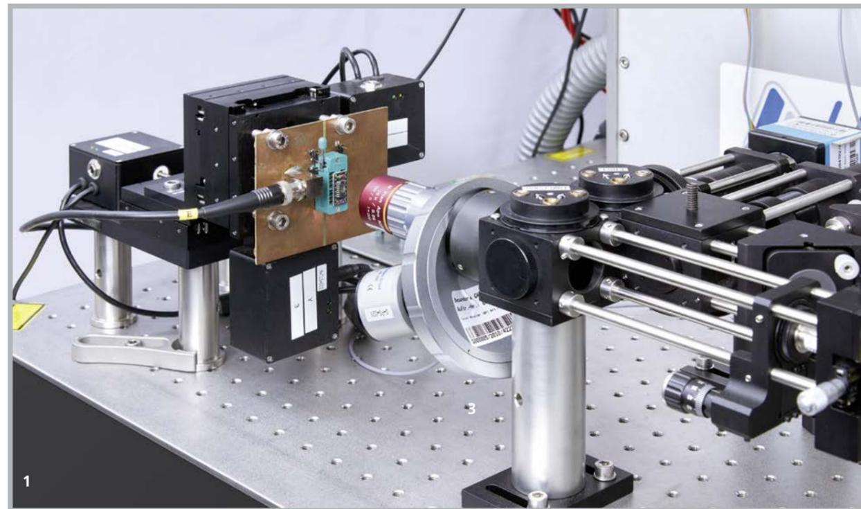
1 Laser-SEE assembly at Fraunhofer INT
